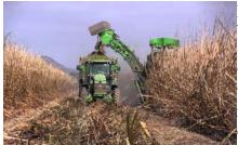
Modern mechanical harvesters cuts the cane at the base of the stalk, strips the leaves, chops the cane into consistent lengths and deposits it into a transporter following alongside. The harvester then blows the trash back onto the field. Such machines can harvest approximately 100 tons each hour.
